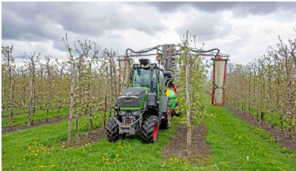
Figure 4. 6 TMS TreeScout, the world’s first fully integrated tractor-mounted sensor for precision orchard management
