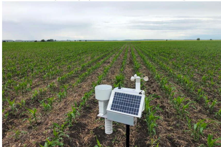
Figure 1.6 Weather and soil monitoring using IoT in corn fields ( https://h2020-demeter.eu/pilots-overview/pilot-cluster-one/iot-corn-management-decision-support-platform/ )
